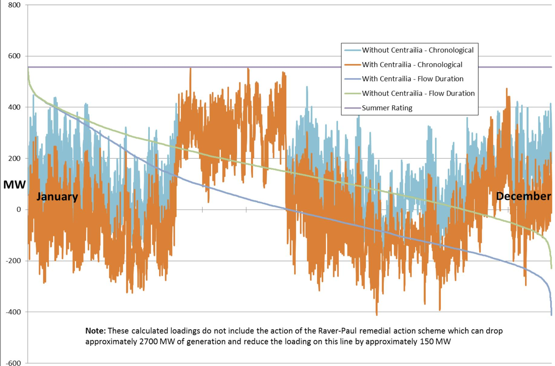
**Note:** These calculated loadings do not include the action of the Raver-Paul remedial action scheme which can drop approximately 2700 MW of generation and reduce the loading on this line by approximately 150 MW
