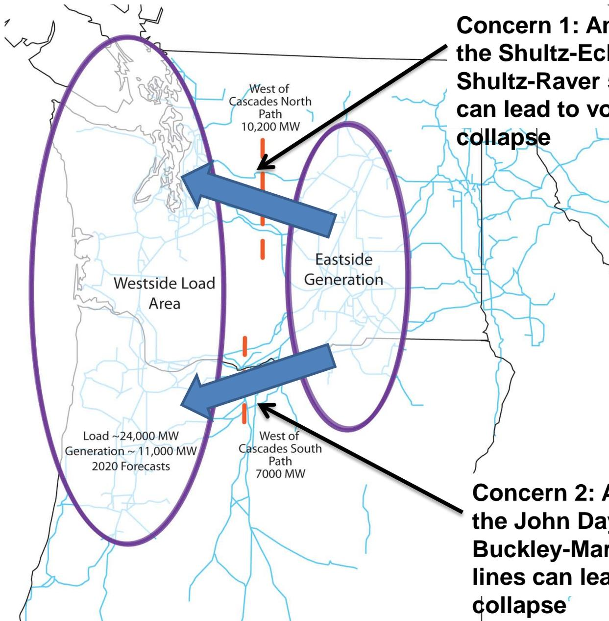
**Concern 1: An outage of the Shultz-Echo Lake and Shultz-Raver 500 kV lines can lead to voltage collapse**
