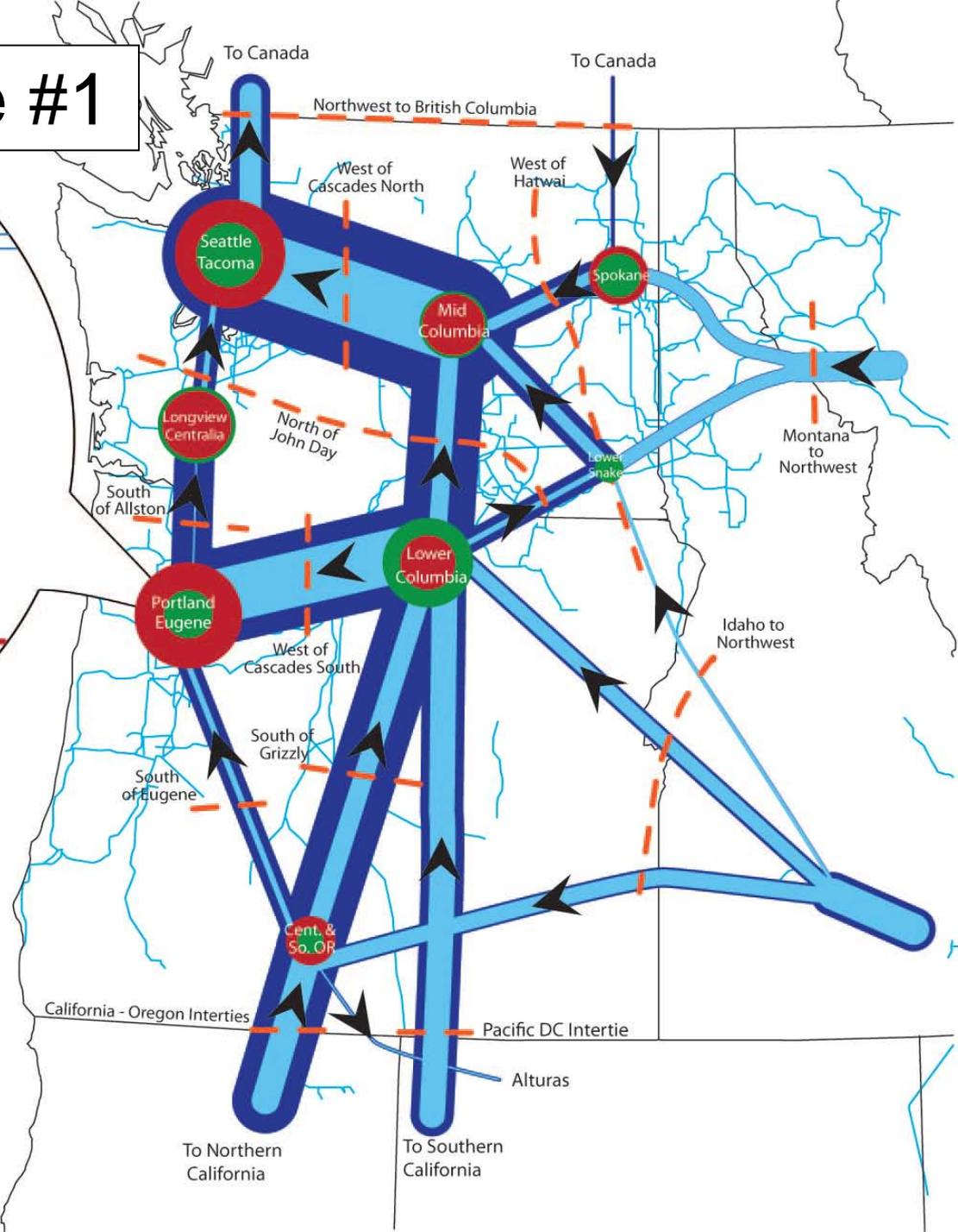
**Concern:** An outage of the Keeler-Pearl 500 kV line can overload the Murray Hill-Saint Mary's 230 kV line and some underlying 115 kV lines
