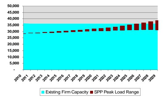
Figure 3-15: Utility Perspective July Capacity Needs Assessment (MW)
