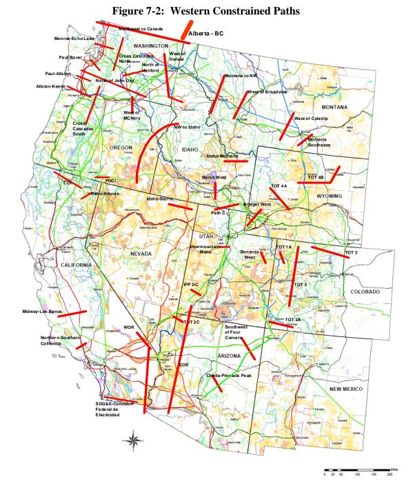
When the loading on an individual path, controlled by individual balancing authorities in coordination with their neighbors (see Chapter 12 for more details on what balancing authorities do) reaches these predefined limits, operators do not allow additional transactions to be scheduled. The system can be said to be congested at that point, though it is not overloaded, but is operating normally.
