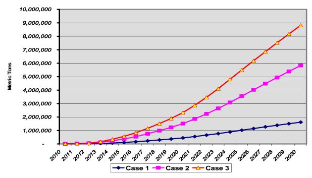
Figure 3-12: Potential Reduction in Tail-pipe CO2 due to Plug-in Hybrid Vehicles
