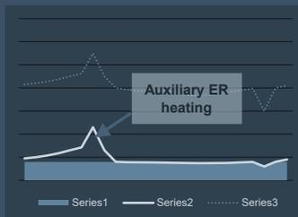
In extreme cold conditions, compressor cannot run and system effectively becomes an ER furnace
