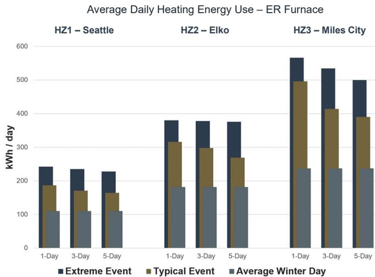
An electric resistance furnace uses 15-40% more energy during an extreme event compared to a typical cold snap.
