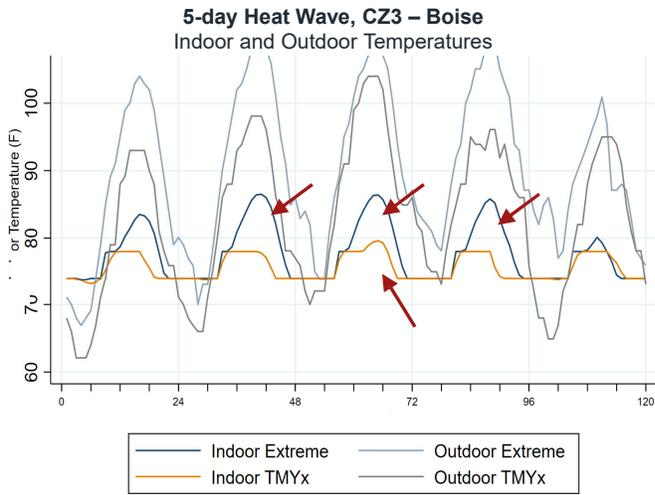
Typical Boise heat wave already stresses 4-ton AC – thermostat temperature slightly exceeded for a few hours on third day.
