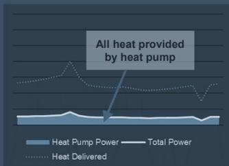
If temperature drops and demand exceeds compressor capacity, ER will make up the difference, reducing efficiency
