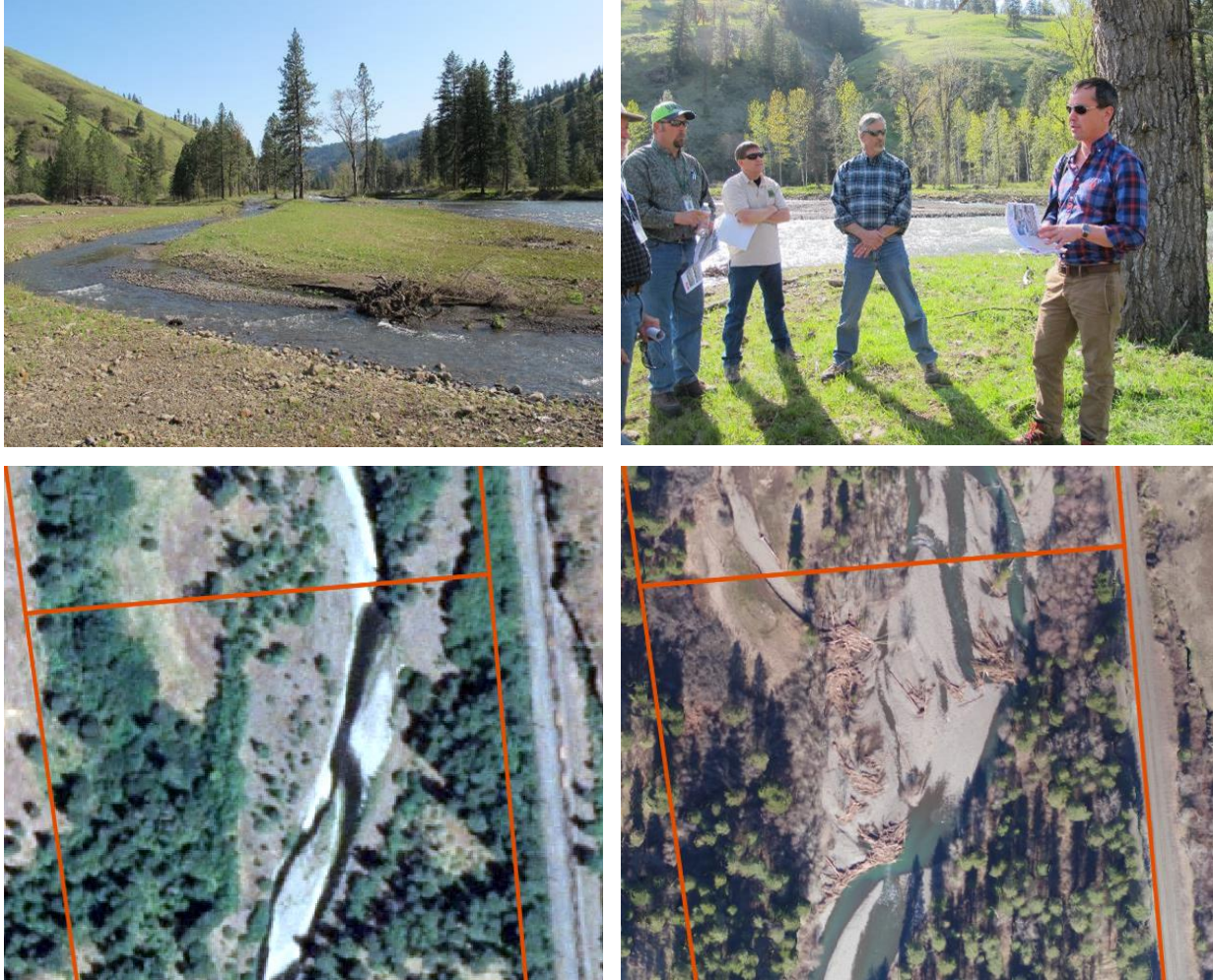
Figure 3.2. Example of floodplain reconnection, Meacham Creek, Umatilla River subbasin, Oregon. (FWP project #1987-100-01, Confederated Tribes of the Umatilla Indian Reservation [CTUIR]). The top two photos are from the ISRP site tour in 2013 with CTUIR staff describing their vision for river restoration, and the bottom two aerial photos show the pre-restoration creek in 2005 and floodplain reconnection and added piles of large wood post-restoration in 2020. (Sources: top photos from the ISRP; bottom photos from CTUIR webpage Meacham Creek Restoration Projects Before and After – click link to use slide bar showing area pre- and post-restoration).
