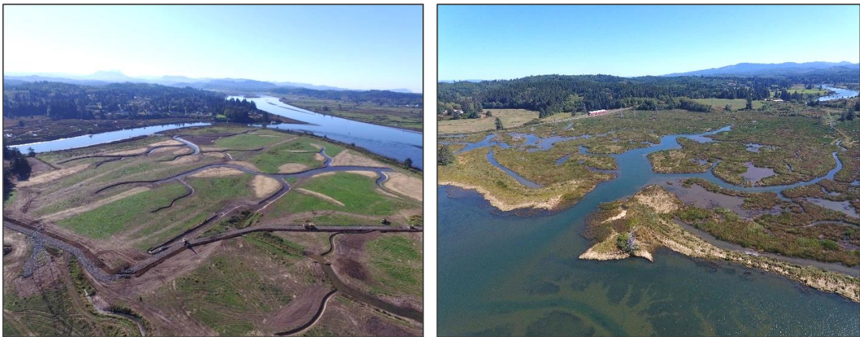
Figure 3.7. Example of dike breaching and tide gate management in the Wallooskee-Youngs estuary restoration project, Astoria, Oregon (FWP project #2012-015-00). This project lowered or removed over a mile of levee and in the process removed 5 tidegates. The project also recreated nearly 10 miles of interior channels from historical data and enhanced LiDAR imagery. The former dairy farm is inundated twice daily providing access to, and organic import from, about 190 acres of tidal marsh. Native plants have germinated, although the vegetation community is still evolving. Top left: Construction in 2017, facing southwest (credit Cowlitz Indian Tribe). Top right: Five years after construction, the largest channel, facing southeast (credit Lower Columbia Estuary Partnership).
