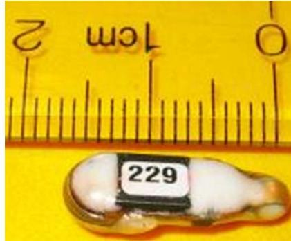
**Figure 5.A.4.1.** JSATS Acoustic Micro-Transmitter with ruler for scale (Photo: courtesy of Pacific Northwest National Laboratory, operated by Battelle for the US Department of Energy).
