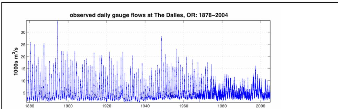
Figure 11: (top) The observed daily average gauge flow at the Dalles, Oregon, from 1878-2004, in m<sup>3</sup>/s. (right) Average daily hydrographs at the Dalles for 1901-1950 (in blue) and 1980-2003 (in red). Note that both figures show the major reduction in daily peak flows, primarily a consequence of hydrosystem development and operations, but also influenced by irrigation withdrawals and climate variations (Naik and Jay 2005).
