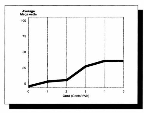
Figure 7-1 Availability and Cost of Transmission and Distribution Efficiency Improvements
