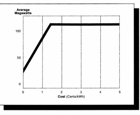
Figure 7-2 Availability and Cost of Hydropower Efficiency Improvements
