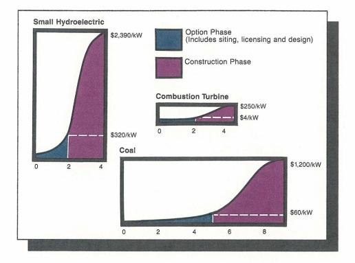
Figure 3-1 Cost and Timing of Optioning and Constructing Resources
