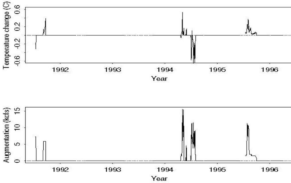
Figure 15. Temperature increase with the existing flow augmentation relative to temperature if Hells Canyon flows were limited to 5000 cfs.
