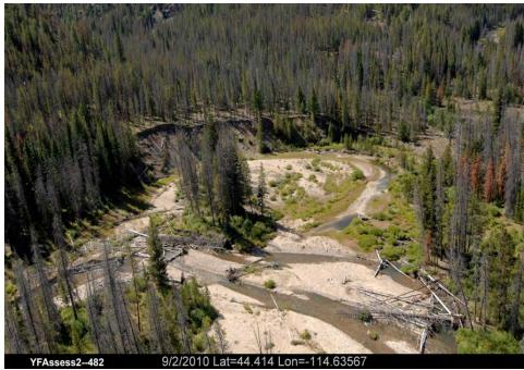
**Figure 23.** View to the southwest near RM 14.9 showing forced alluvial channel variability. *Wood complexes influence variability in channel processes and habitat complexity. Lake and glacial outwash deposits (eroded high bank in the background) are common in this geomorphic reach and provide sediment inputs of predominantly gravel to fines.* Bureau of Reclamation photograph by Dave Walsh, September 2, 2010.
