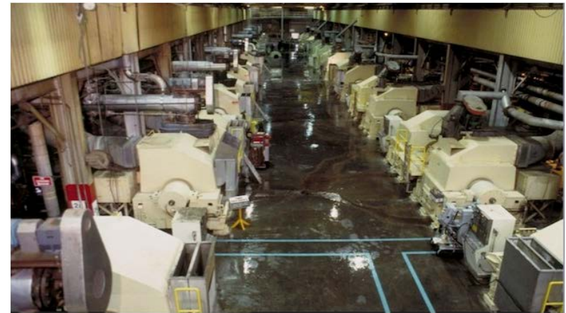
Northern Pacific Paper Corporation (NORPAC) in Longview, Washington is a giant consumer of electricity. NORPAC uses huge thermal mechanical pulping refiners, shown here, that are driven by over three dozen 6,000-horsepower motors that use 150 MW to produce 1,600 tons of paper per day. But some of these refiners don't have to be running at any particular time, so can be shut down to lower demand in response from a power company request because of a demand spike elsewhere. This is the core of the Demand Response program to increase energy efficiency in the Pacific Northwest and reduce the need to build new energy plants, wind farms or pipelines. Source: Energy Northwest
