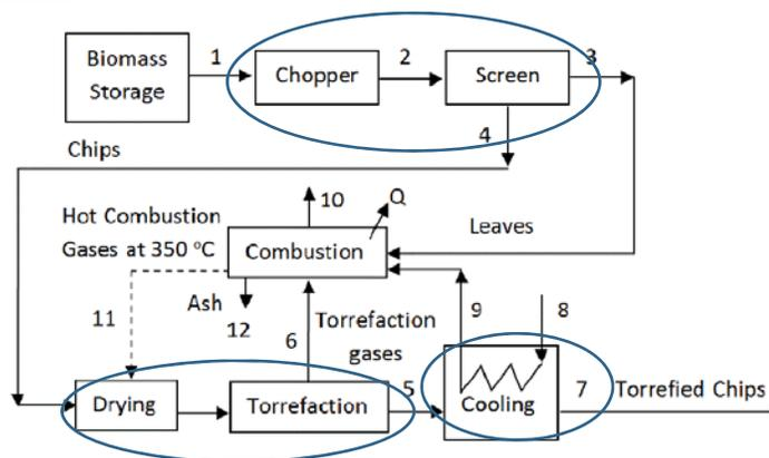
Figure 3 Conceptual design of a proposed torrefaction process proposed (Bergman et al. 2005).
