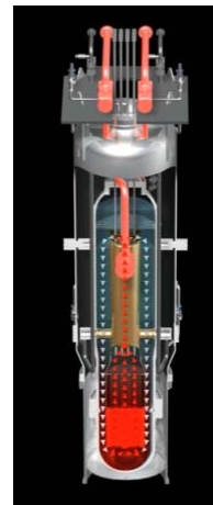
primary coolant flow path
