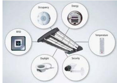
Luminaire Level Lighting Controls
