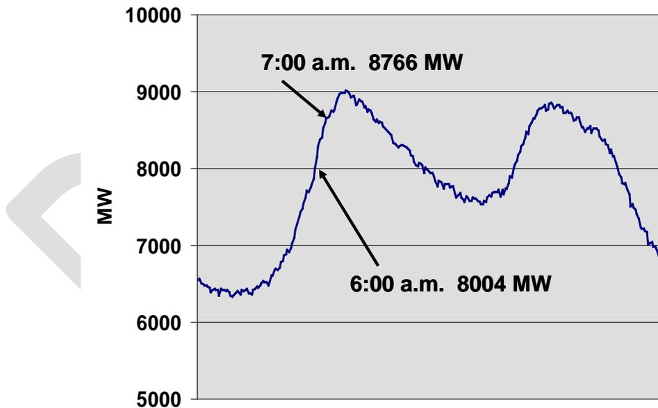
A balancing authority has to deal with a load ramp of, for example, 762 megawatts over the course of an hour, using the generation under its control in its own balancing area. At the same time, it must deal with any imports or exports that have their own time pattern for adjustment. Scheduling between balancing authorities in WECC is generally done in one-hour increments, with the schedules ramping in across the hour, from 10 minutes before the hour to 10 minutes after the hour.
