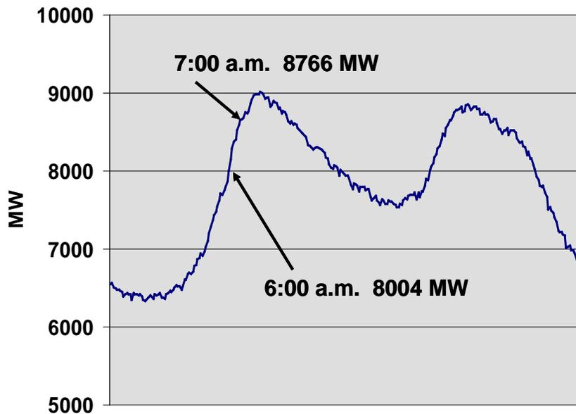
A balancing authority has to deal with a load ramp of, for example, 762 megawatts over the course of an hour, using the generation under its control in its own balancing area. At the same time, it must deal with any imports or exports that have their own time pattern for adjustment. Scheduling between balancing authorities in WECC is generally done in one-hour increments, with the schedules ramping in across the hour, from 10 minutes before the hour to 10 minutes after the hour.
