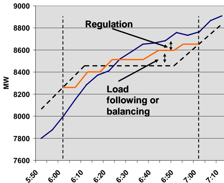
\*Dashed line shows scheduled generation, solid blue line shows actual load and orange line in between separates the AGC regulation from load following actions.
