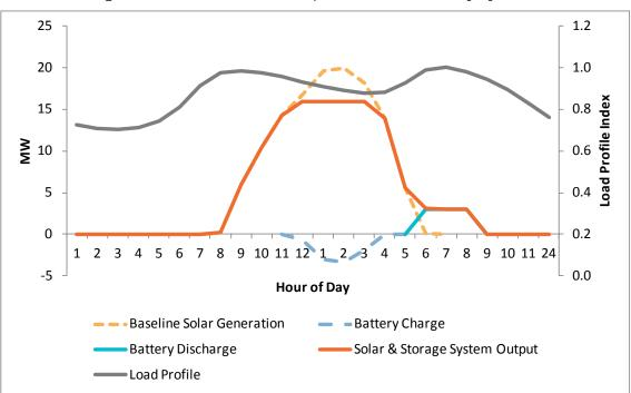
Figure H - 4: Modeled Example of Solar + Battery System
