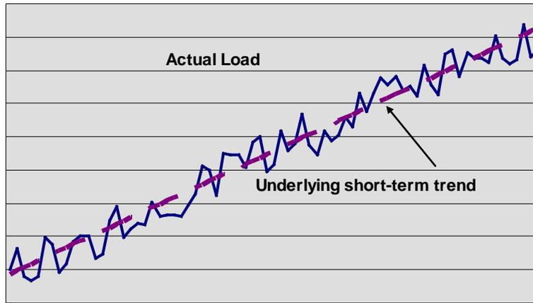
Figure 10 - 8: Illustration of Hourly Scheduling with Load Following\*
