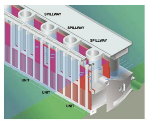
The design at Wells Dam enables the spillway, on top of the turbine intakes, to function as an efficient bypass system.
