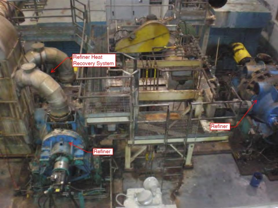
Hydraulic Starter Motor for Refiner & 12000 HP Motor
